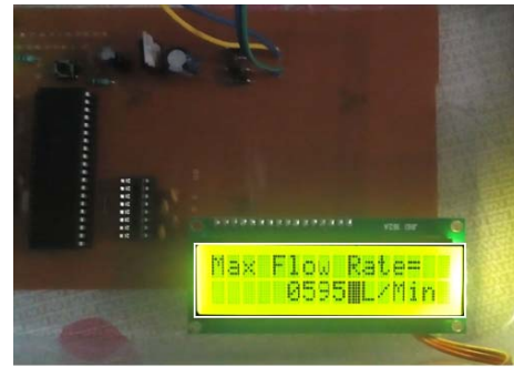
Fig. 6 Result2- Maximum flow rate = 595L/Min
