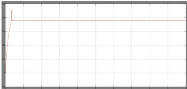
Fig 11: Constant DC link voltage (380V)
